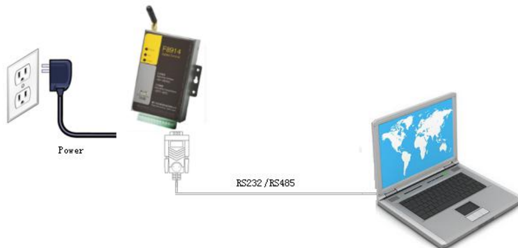
Figure 3-1 F8L10T configuration connection with PC
