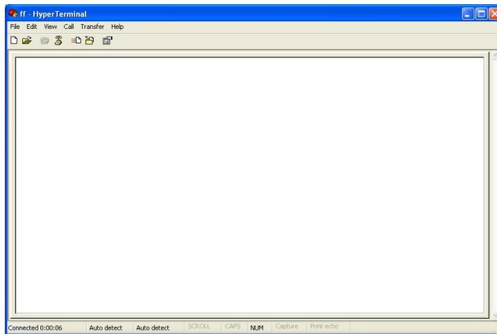
6. Re-power NB-IoT Terminal, put mouse focus on the Hyper Terminal and press “s” key continuously until NB-IoT Terminal enter configure state as following.
