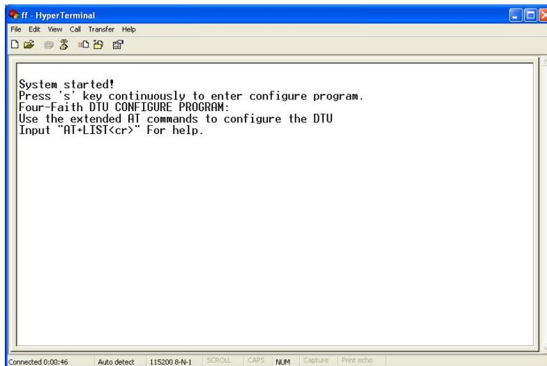
7. NB-IoT Terminal has entered configure state, you can configure the parameters through AT command.
