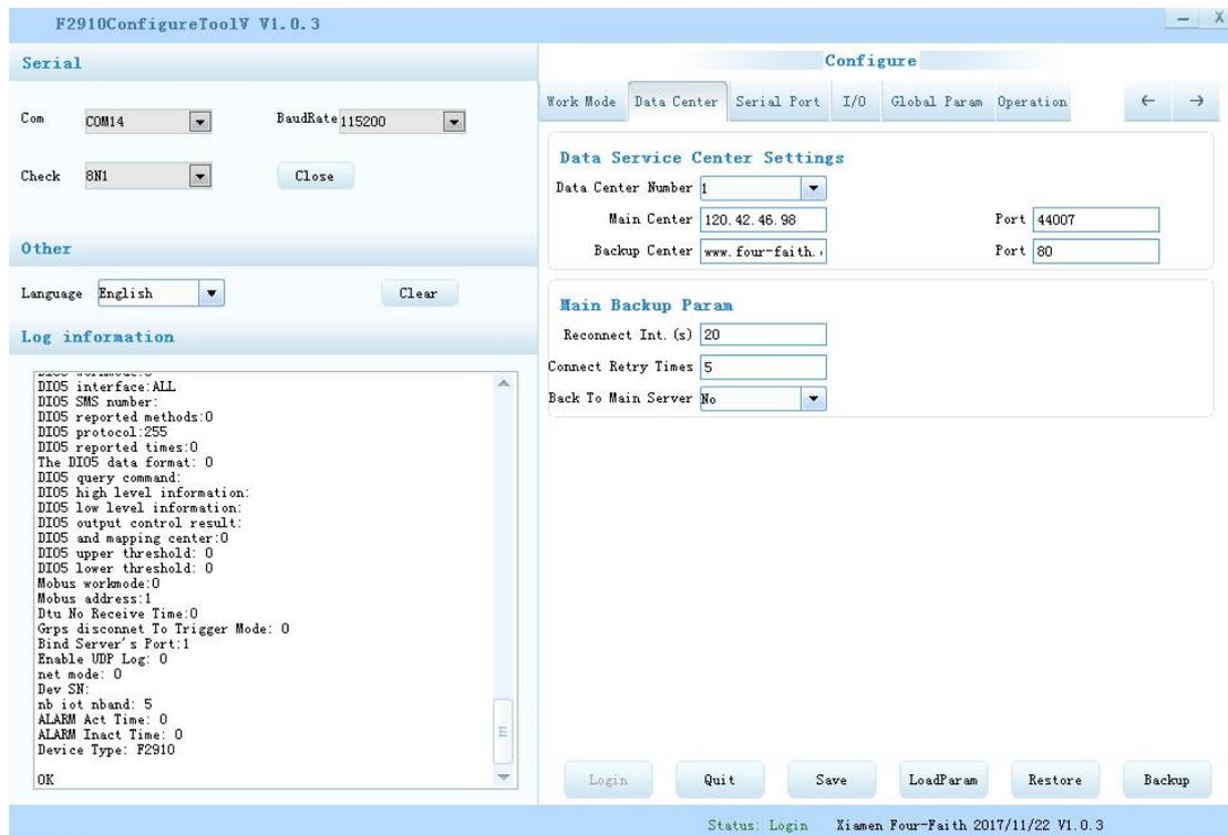
After Re-power NB-IoT Terminal, The configure tool will make it enter configure state. The software will load current settings from NB-IoT Terminal and displays on the right configure columns at the same time. It's now ready to configure.
